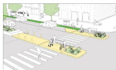
**Medians and Refuge Islands.** These roadway elements provide physical separation between opposing vehicle lanes, and narrow roadway widths to reduce vehicle speed. Median islands are typically landscaped to improve the aesthetics. They can provide a “gateway” appearance when placed at the entrance to a neighborhood, and are often combined with textured pavements. They can also be used to provide a pedestrian refuge area in the center of the roadway by providing a gap in the island.
