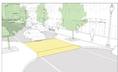
**Speed Tables.** Speed tables are long, flat-topped raised areas on roadways that span across the width of a travel lane. They are similar to speed humps but with a longer flat surface, providing a smoother, more gradual rise and descent for vehicles. They are often combined with crosswalks, creating raised crosswalks that enhance pedestrian visibility and safety.
