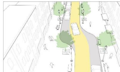
**Chicanes and Lateral Shifts.** These features include a series of curb extensions that alternate from one side of the street to the other, forming S-shaped curves that essentially narrow the roadway width and create an effect that slows down traffic.
